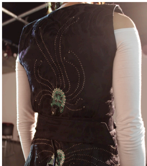
Figure 3 The back zone and the belt zone. The vibrotactile elements lie underneath the area between two connector endings emanating from each of the central boards.
