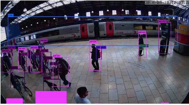
Figure 2 Realtime Object Detection on the Platform
