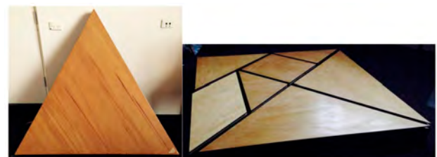
Figure 1 Left: One of Cullen's four identical Vernus Pressure-Sensitive Floors, built in 1972. Right: The Terpsichora Pressure-Sensitive Floors, built in 2015. 7 platforms forming a tangram shape, each with one sensor underneath, responding to movement
