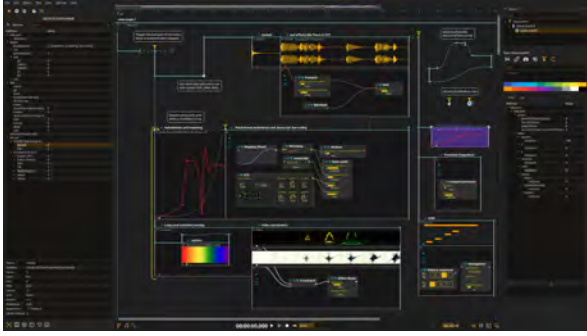
Figure 2: A screenshot of ossia score , showing the main system for authoring scores with the visual language of fig. 1. On the left, a tree view shows the OSC addresses to which the score can speak. On the right, an inspector allows to edit the properties of selected elements. The score is in the center.
