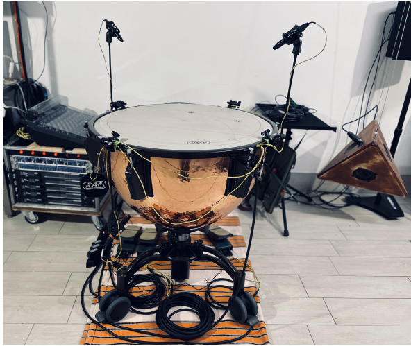
Figure 1. The Tempo instrument at LEAP laboratory: Adams Revolution 29” hand-hammered copper timpani with tetrahedral microphone array, neodymium magnet pairs on the membrane, and geometric tracings of the Due Lune map. On the left, the SSL BiG SiX mixer and the power amplifier driving the induction system; on the right, a S.T.ONE tetrahedral loudspeaker.
