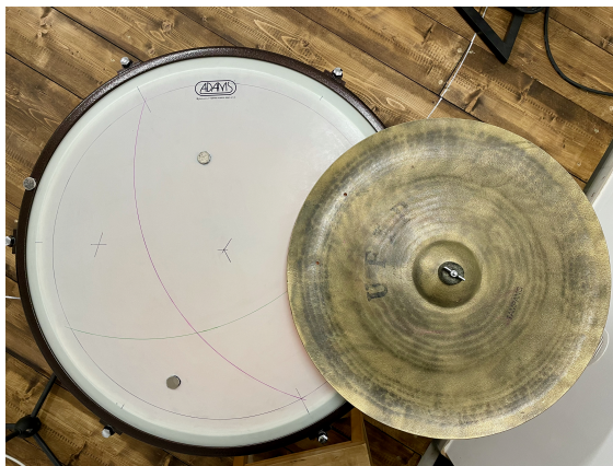
Figure 6. Top view of the freshly traced Due Lune (Two Moons) cartography on the membrane, with neodymium magnets still off-position. The four constraint points arise from distinct geometric intersections: \alpha from lune and circumference, \beta between the two lunes, \gamma on an external triangular intersection axis, \delta from circumference and lune—replicating the theoretical map of Fig. 4.
