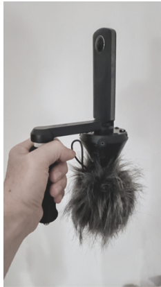
Figure 2. Synchronized recording setup for a Soundspace-Sequenz : first-order Ambisonics (FOA) microphone and 360° video camera used for re-listening and positional verification.
