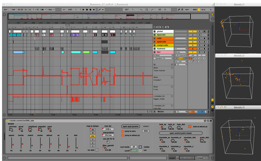
Figure 1. Screenshot from Max for Live environment showing breakpoint functions used to control flocking behaviors of virtual sources in a piece using spatial audio. On the right side of the screen are OpenGL visualization of point locations generated by the many parameters contained within the algorithm. In a more symbolic notation environment, the parameters of the resulting rendering would be representational of their function.
