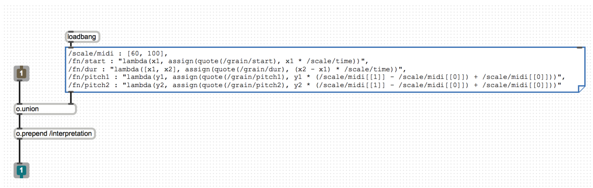
Figure 5. Example of storing interpretations of graphic information contained in the SVG file in Odot lambda functions. Here, the function describes a process of interpretation where the x1 value indicates the start time, scaled to a given time constant, and the duration is the horizontal span of the object.
