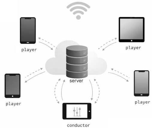
Figure 1. Local-network setup with conductor and multiple player devices connected to a central server.
